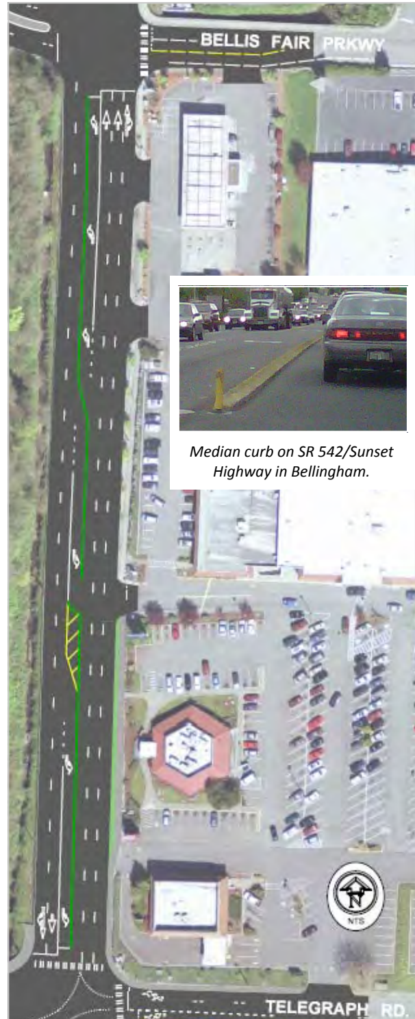
An illustration of where turns might be located when the center-turn lane is replaced with curb.
